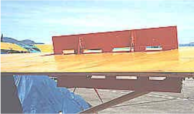
This photo shows the spoilers on an Air Cadet glider.
