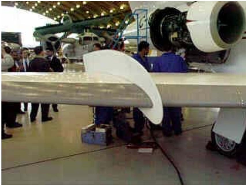
This photo shows a wing fence on a Falcon jet in the BCIT hangar.
