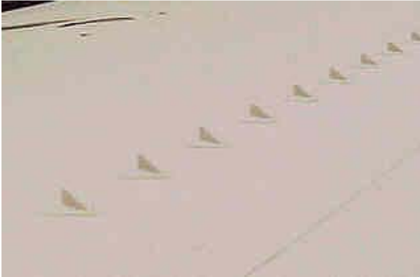
This row of vortex generators are along the wing of a Citation X
