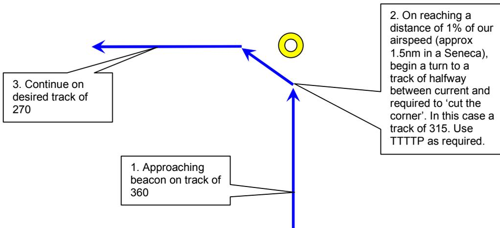
A commercial turn means that we do not actually fly directly over a waypoint, but anticipate arriving and turn onto a track to intercept our new required track, as shown in figure 8.
