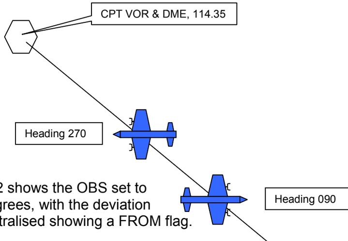
Figure 2 shows the OBS set to 140 degrees, with the deviation bar centralised showing a FROM flag.
