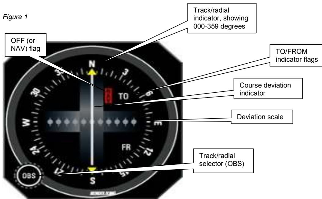
Figure 1 shows the VOR display. The key features are identified, with further explanation below:
