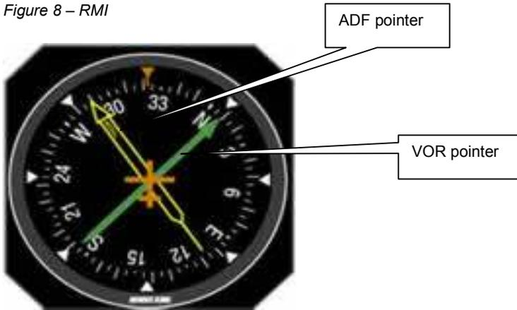
Figure 8 shows a typical RMI. Again, slaving should be checked prior to and during use. The example shows the aircraft with a track of 010 to the VOR, on the 190 radial. The NDB needle (ADF) shows a QDM (magnetic bearing to) of 290, and a QDR (magnetic bearing from) of 110.
