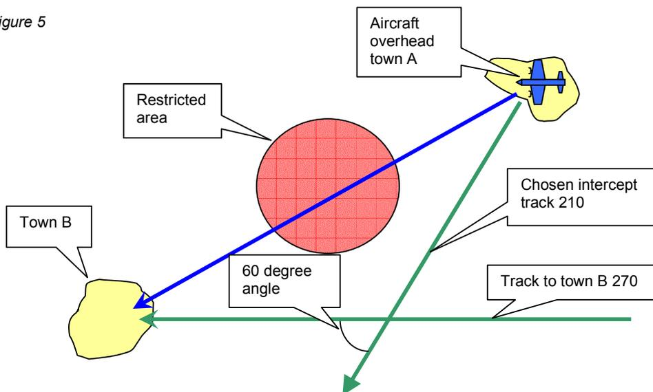
From overhead town A, we wish to fly to town B, but there is a restricted area on the direct track, which we cannot overfly. We must therefore fly around, and in order to do so we decide to fly inbound to town B, with a 60 degree intercept of that track from our current position. This clearly involves an initial track of 210 to achieve this intercept. In doing this we have answered all three of the above questions: where am I; where do I want to go; how do I get there.
