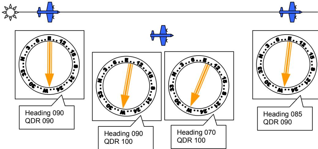
This time as the aircraft is blown off track the tail of the needle indicates an increasing QDR. The error is noticed when the QDR is 100. To correct we WANT less QDR, so must STEER less. As we want 10 degrees less QDR we should steer 20 degrees less heading, making 070. As the needle moves back to show a QDR of 090 we apply a compromise heading of 085 to prevent further errors.
