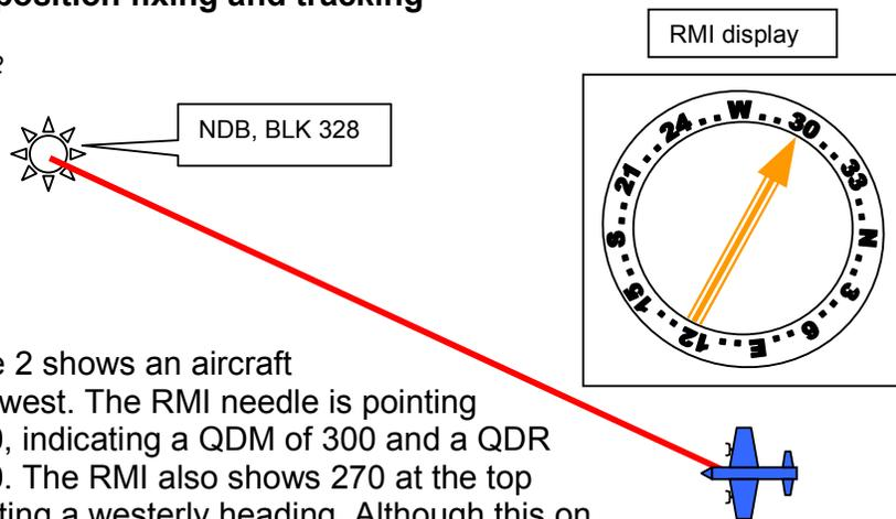
Figure 2 shows an aircraft flying west. The RMI needle is pointing to 300, indicating a QDM of 300 and a QDR of 120. The RMI also shows 270 at the top indicating a westerly heading. Although this on it's own does not fix the aircraft's position, linked to a DME/VOR or by cross-cutting a 2<sup>nd</sup> NDB it can be seen that position fixing is fairly straightforward.
