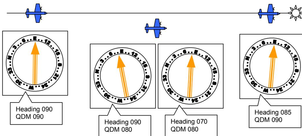
As the aircraft is blown off track the ADF pointer begins to move. In the example the error is noticed when the QDM has fallen to 080. We now WANT more QDM, so must STEER less. In order to correct we double the error. This
