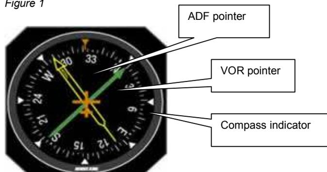
Figure 1 shows a typical ADF display. The compass card rotates automatically with the HSI (see VOR notes), showing aircraft heading at the top. The yellow needle points to the beacon, with the head showing QDM (magnetic bearing to) and the tail showing QDR (magnetic bearing from). It is quite common to also have a green VOR pointer on the display also, which is discussed in the VOR notes).
