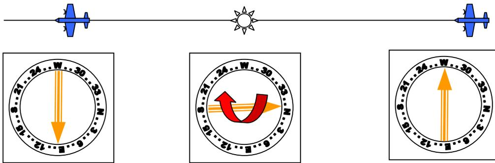
Figure 3 shows the situation in zero wind conditions. Initially the aircraft has a heading of 270, with a QDM of 270. As it passes over the beacon the needle will flip. The rate at which it turns depends on accuracy of tracking. Once through the overhead the instrument shows a heading of 270, and now a QDR of 270 (QDM 090).
