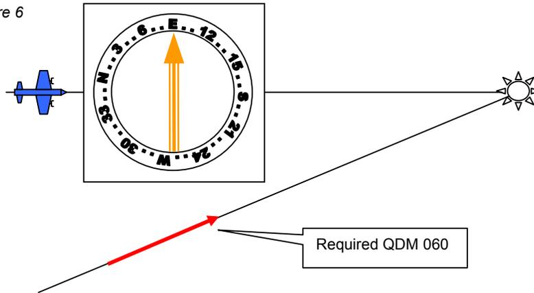
Figure 6 shows an aircraft tracking towards an NDB with a QDM of 090. A track of 060 is now required:
