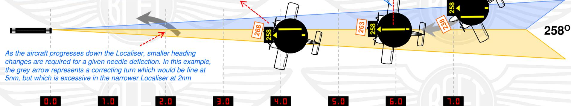
• The "golden rule" for flying the Localiser is to action corrections on the AI with reference to the HSI
